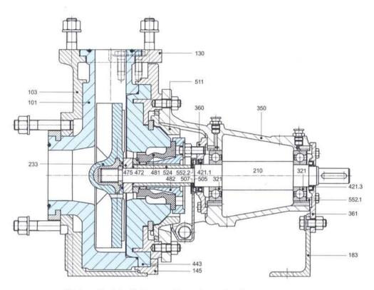
The type illustrated is the one with semi open impeller. Only order spares according to the relevant parts list.
