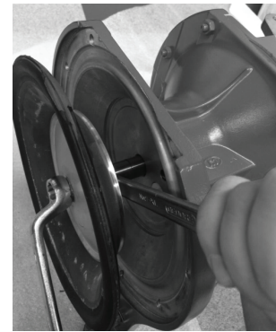
Pic. 5: Hold it in place with wrench
